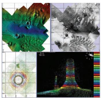
Imaging of pillars and sediment features of a bridge crossing.
